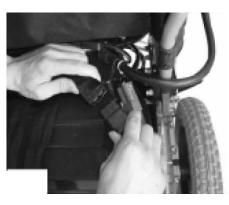
Assemble the footrest on the wheelchair and lock it by latch.
