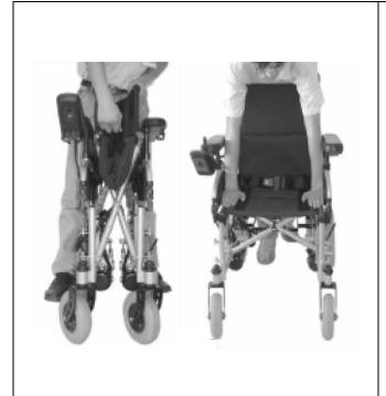
Press the seat tubes down with both hands and make sure the crossbar tubes are tight and locked.
