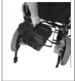
**5** Connect the two batteries together using the red battery connectors.
