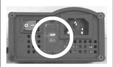
10 Ensure that the 115V/230V switch on the product's battery charger is set to 115V. If the switch is set to 230V, the scooter will not charge properly.
